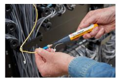
The award winning FiberLERT from Fluke Networks is the first live optical fibre detector for resolving the cause of communications failure in fibre optic networks. The pocket sized tool enables the effective troubleshooting of invisible near infrared (850nm-1625nm) wavelengths used in fibre optic communication, with the quick identification of failures in a port, polarity and transceivers.
