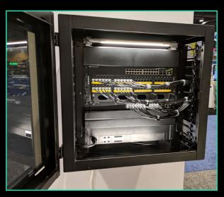
We are seeing edge computing installed in managers offices, hallways, back rooms, and even in customer facing areas, whether at eye level or on poles above. This means that the computing equipment needs to be housed in a smaller type of cabinet.
