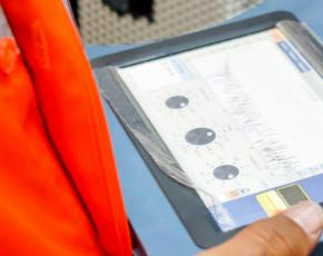
conducting light source and power meter testing of fibre optic cables. Your test plan may also stipulate optical time domain reflectometer (OTDR) testing and further useful information to be included within the final project documentation.
